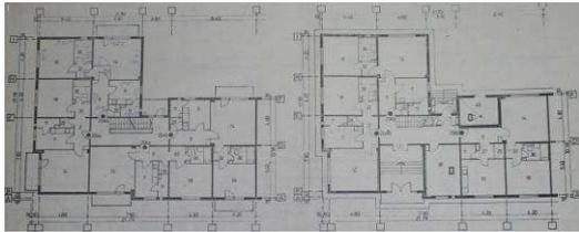
Figure 3. The standard project T1340-IPCT; horizontal section of the current floor on the left, horizontal section of the ground floor on the right
